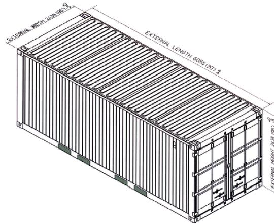
Figure 6 - 20 ft ISO Dry Cargo Container ([www.seabox.com](http://www.seabox.com))
