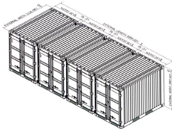
Figure 7 - 4 Quadcons Configured as Sea Container ([www.seabox.com](http://www.seabox.com))
