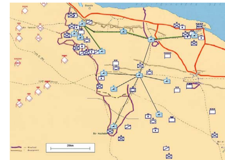
Figure 3: CLARION screenshot showing forces lay out with commodities flowing along Arcs to Dumps. Here fuel has been assigned the colour green and is shown moving from the logistic Dumps to Dumps which are closer to the combat units requiring re-supply of fuel.
