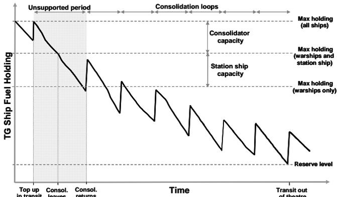
Figure 3. Example of TG fuel holding as a function of time with minimised tanker capacities.
