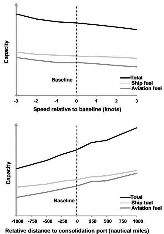
Figure 5. Relationship between capacity requirements and consolidator speed (top) and distance to port (bottom).
