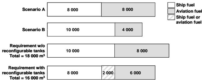
**Figure 6.** Fuel capacities (in m<sup>3</sup>) required by two notional scenarios. A tanker with reconfigurable tanks can support either scenario with 16,000 m<sup>3</sup> of usable capacity.
